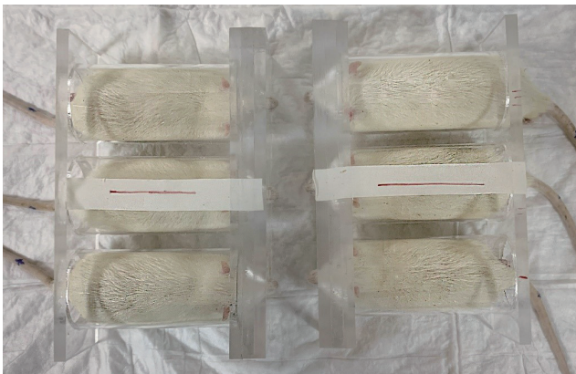
Fig. 2. The device for whole-brain radiotherapy and placement of the rats.
