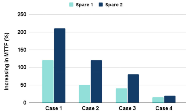
FIGURE 10 The effect of failure conditions and redundancy levels on network MTTF.
